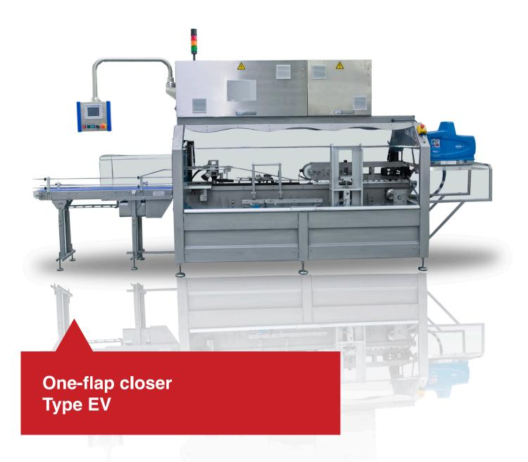
The formed cartons, which are made of full or corrugated cardboard, are fed into the closing machine. The lateral dust flaps are folded in by a folding device and a servo-driven flap-insertion device. Optionally, glue points are applied onto the dust flaps. The lid is bent by means of a lid device.
