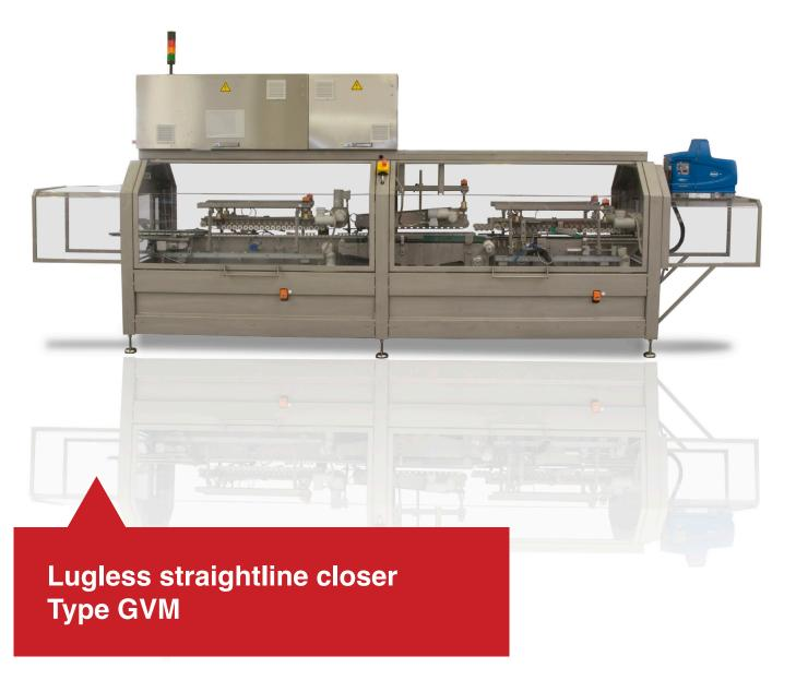
The cartons are continuously fed into the running machine, thus an accumulation can be prevented. The cartons are fixed between upper and lower belts for further transport. Glue is applied on the front flap; the flap is bent and pressed on. The cartons are turned by 90° with the help of a belt-driven mechanical turning device. After glue has been applied on the lateral flaps, the flaps are bent and pressed on and the closed carton is fed out of the machine.
